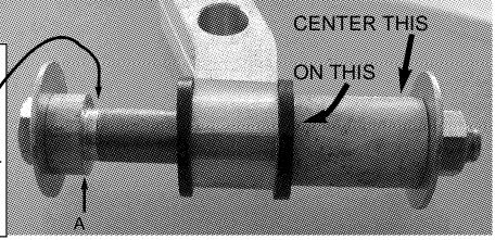
**6.** Keeping the nut from rotating screw the bolt in clockwise. This will push the replacement bronze sleeve into the urethane bushing and the old bronze sleeve will be ejected into the receiver. Keep the replacement bronze sleeve lubricated. Depth gauge will set the sleeve at the proper depth when edge A touches the urethane. At this point remove the tool and discard the old bronze sleeve. Important: Keep the receiving sleeve centered on the other side of the urethane bushing.
